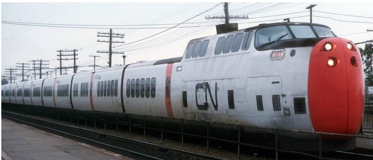
*The UAC Turbo Train operated in Canada between 1968 and 1984. It was an early high-speed gas turbine train and was also one of the first tilting trains to enter service.*
