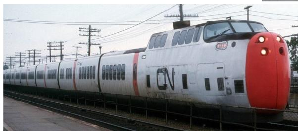
The UAC Turbo Train operated in Canada between 1968 and 1984. It was an early highspeed gas turbine train and was also one of the first tilting trains to enter service.
